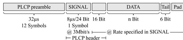
Figure 3. PDU packet format in IEEE 802.11p
