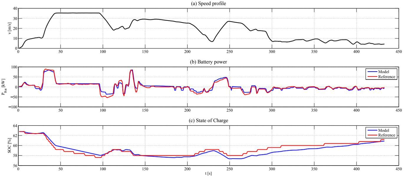
Figure 4. Validation results of freeway test drive
