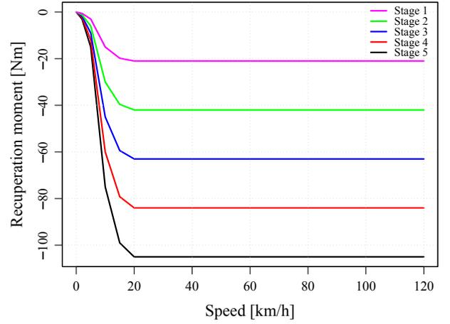
Figure 2. Speed-dependent recuperation moment  $M_{\text{Recu}}$  for each recuperation stage
