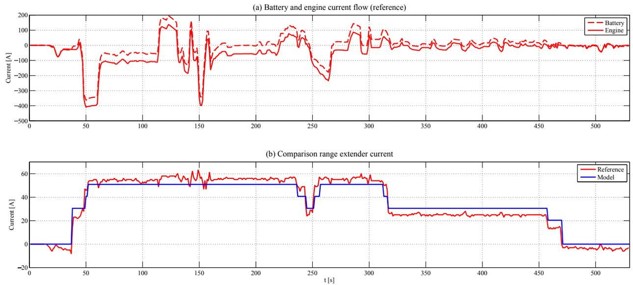
Figure 5. Validation results of range extender module
