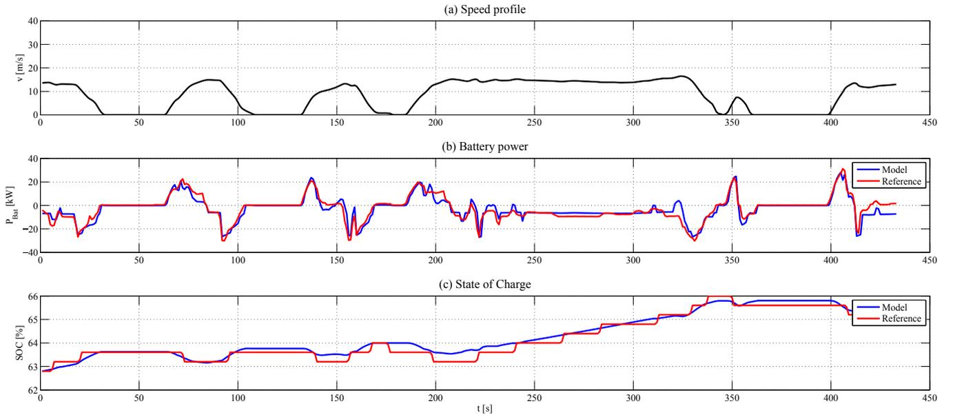
Figure 3. Validation results of the urban test drive
