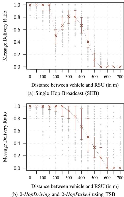
Fig. 3. Combined MDR of MAP and SPAT across all approaches. Plotted is the median MDR depending on the distance to the traffic light RSU. Error bars extend from the 25% to the 75% quantiles.
